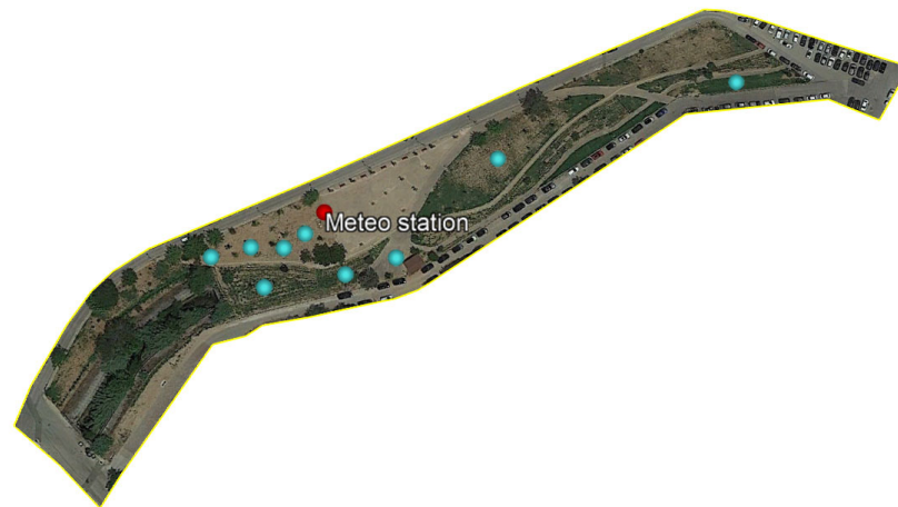
Figure 2. Points inside the UGS where infiltration measurements were taken for the estimation of the unsaturated hydraulic conductivity of the soil (4 points for dry bare soil, 3 points for shrubs and 1 point for grass) (base map by Google Earth, Image © 2022, Google, Maxar Technologies).
