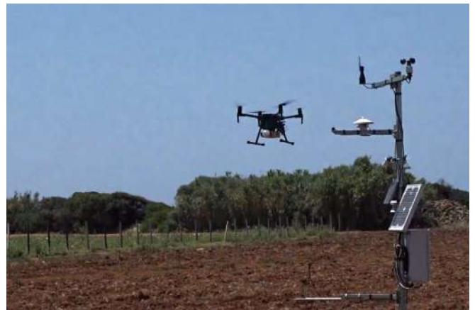
Figure 14: Monitoring water status through combined use of meteorological station and drone (© Agricultural University of Athens).
