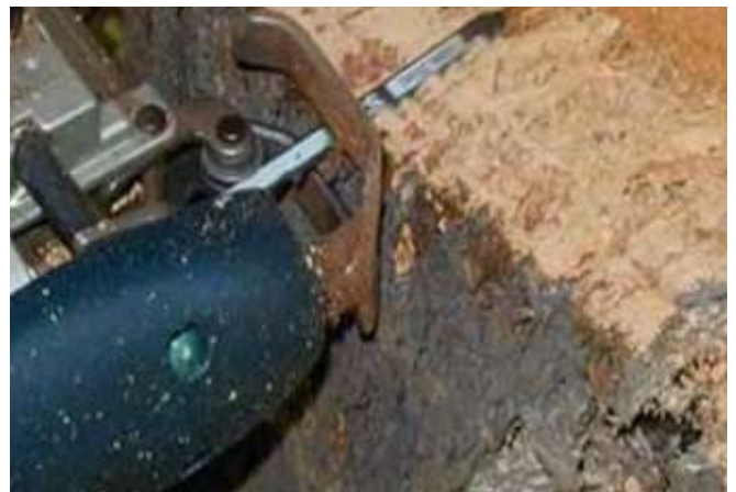
Figure 15: The cork debarking machine tested in Sardinia includes sensors capable of guiding it by measuring the different hydration of phellogen and cork (© The publication "The cultivation of cork oak").
